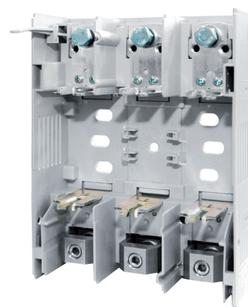
RBK 1VD-M for installation on mounting plate, picture of fuse switch disconnector without fuse links cover and terminal shrouds, top cable terminal - M screws, bottom cable terminal - V-clamps, (RBK 1 VG-M - bottom cable terminal - M screws, top cable terminal - V-clamps)
