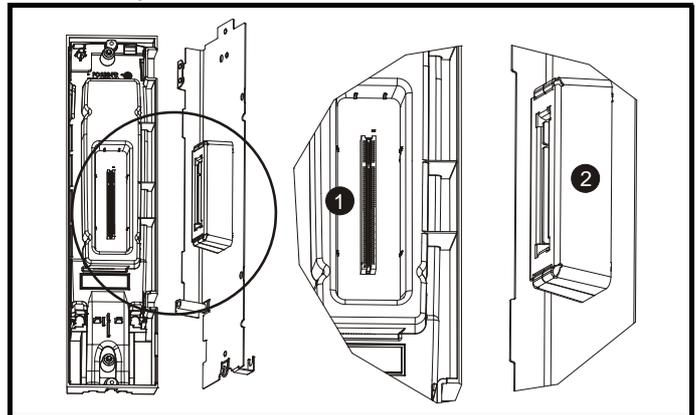
Ensure that the connector on the back of the control master/slave pod (1) is securely fitted to the power module metal base plate connector (2).
