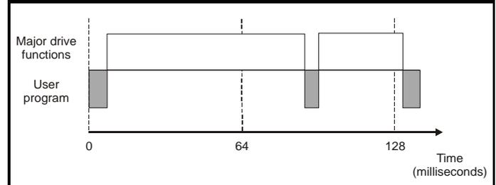
The user program is scheduled for a short period approximately once every 64ms. The time for which the program is scheduled will vary between 0.2ms and 2ms depending on the loading of the drive's processor.
