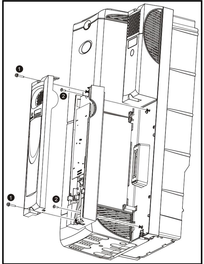
1. In order to expose the mounting holes, remove the control slave pod cover. This is done by undoing the screws highlighted and pulling the cover off.
