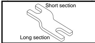
The mounting bracket must be installed in the correct orientation with the long section inserted into or attached to the drive and the short section is attached to the back plate. Figure 5-23 shows the orientation of the mounting bracket when the drive is surface and through-panel mounted.
