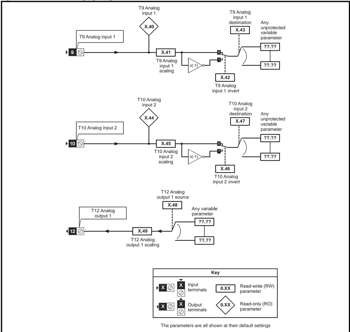
Figure 13-30 SM-I/O Plus digital logic diagram 1
