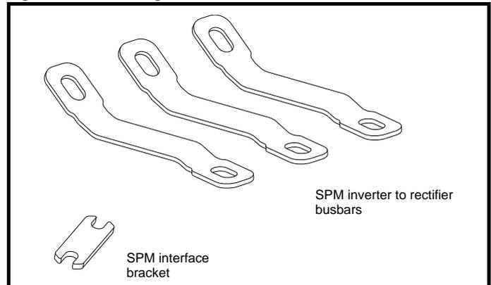
The SPM interface bracket should be connected first, followed by the SPM inverter to rectifier busbars, to the appropriate terminals as shown in Figure 5-13.
