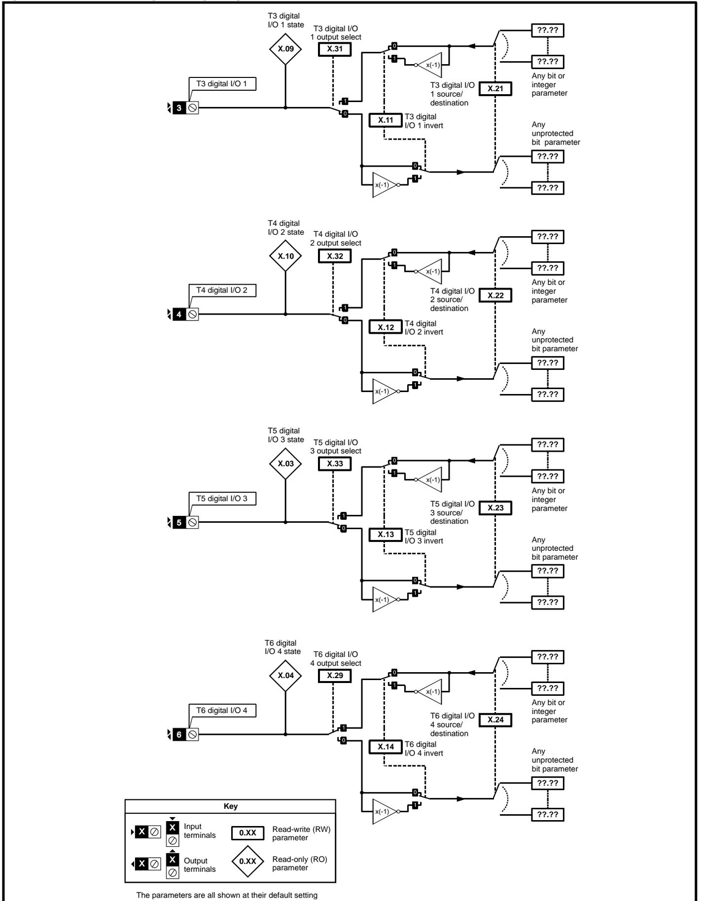
**Figure 13-36 SM-I/O PELV digital input logic diagram**
