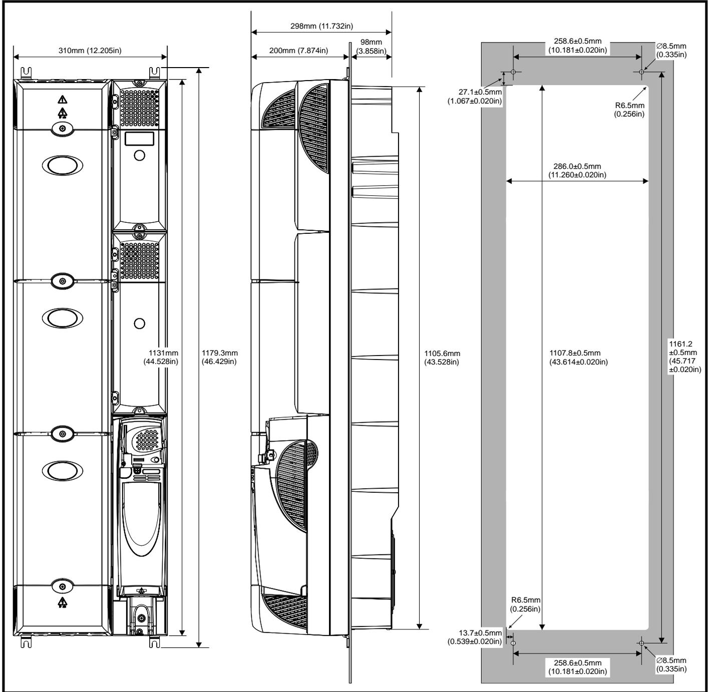
**Figure 5-19 Through-panel mounting the Unidrive SPMD**
