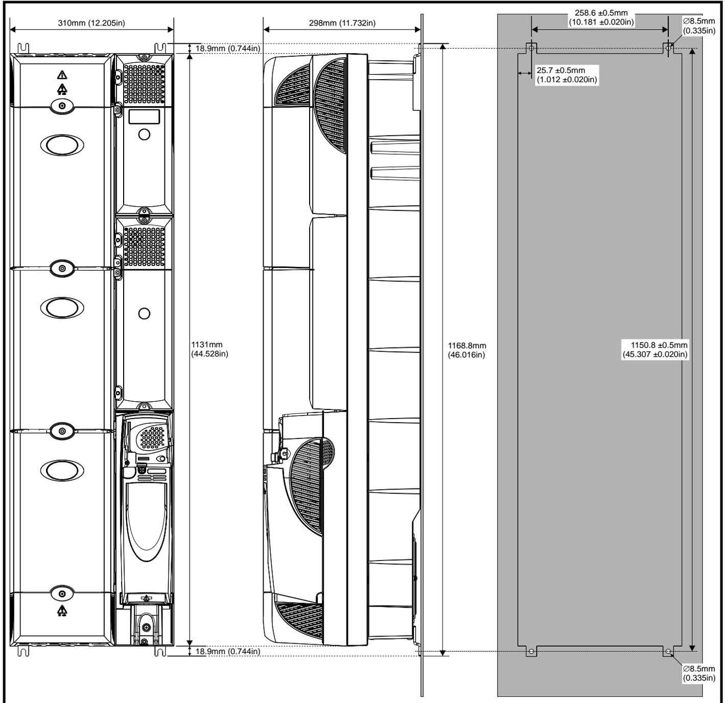
**Figure 5-15 Surface mounting the Unidrive SPMD**
