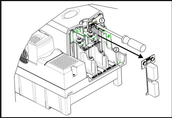
Loosen screws (1). Remove EMC filter in the direction shown (2).
