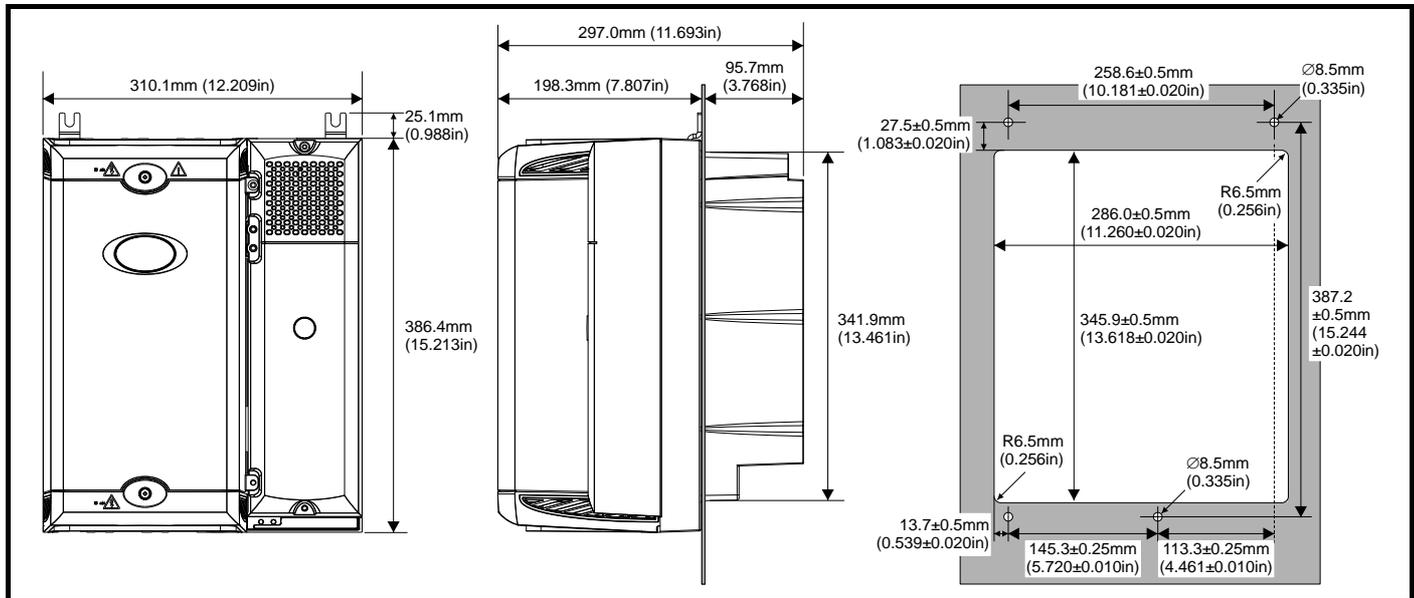
**Figure 5-21 Through-panel mounting the Unidrive SPMD with SPMC/U (rectifier) and docking kit**
