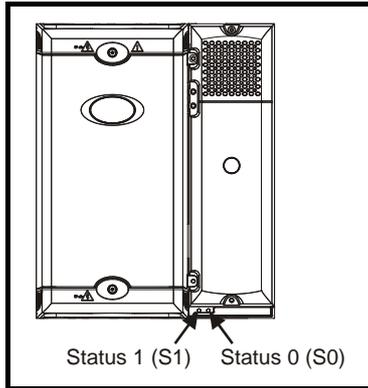
The STATUS LEDs S0 and S1 mirror the status outputs and are encoded as follows:
