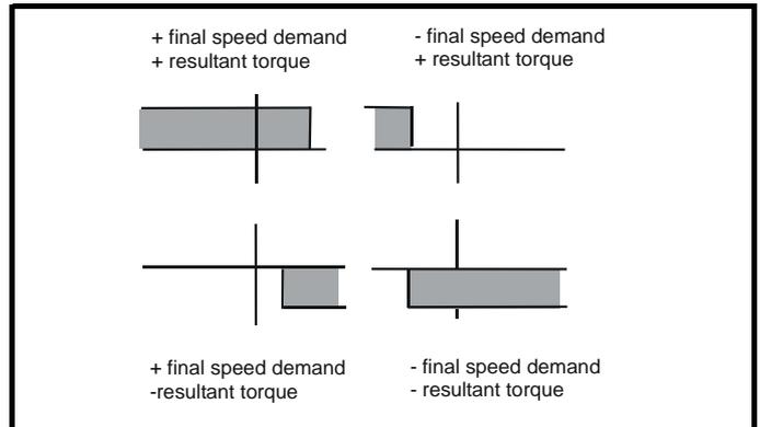
This mode of operation can be used where torque control is required, but the maximum speed must be limited by the drive.
