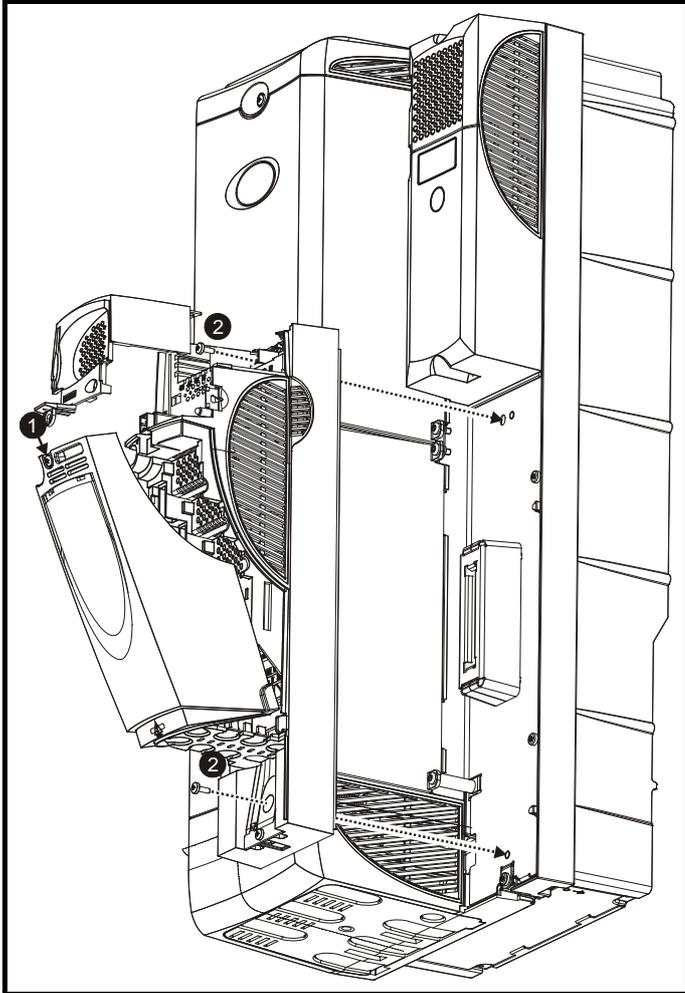
1. In order to expose the top mounting hole, the terminal covers need to be removed. This is done by undoing the terminal cover screw highlighted and then removing the two plastic covers.
