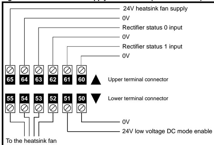
The heatsink fan supply requirements are as follows:
