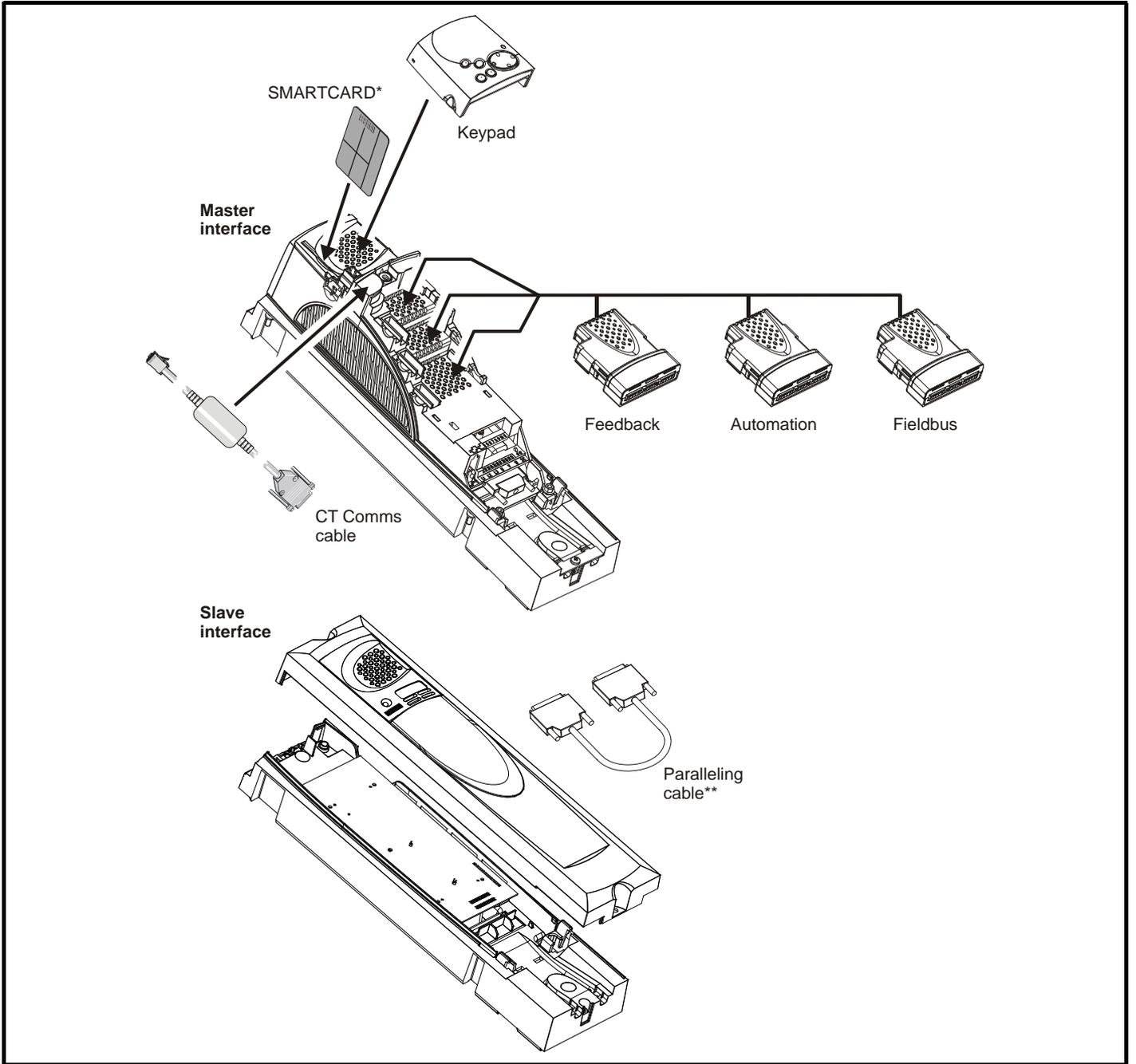
\* A SMARTCARD is provided as standard. Only one SMARTCARD can be installed at any one time. For further information, refer to Chapter 11 SMARTCARD operation on page 149.
