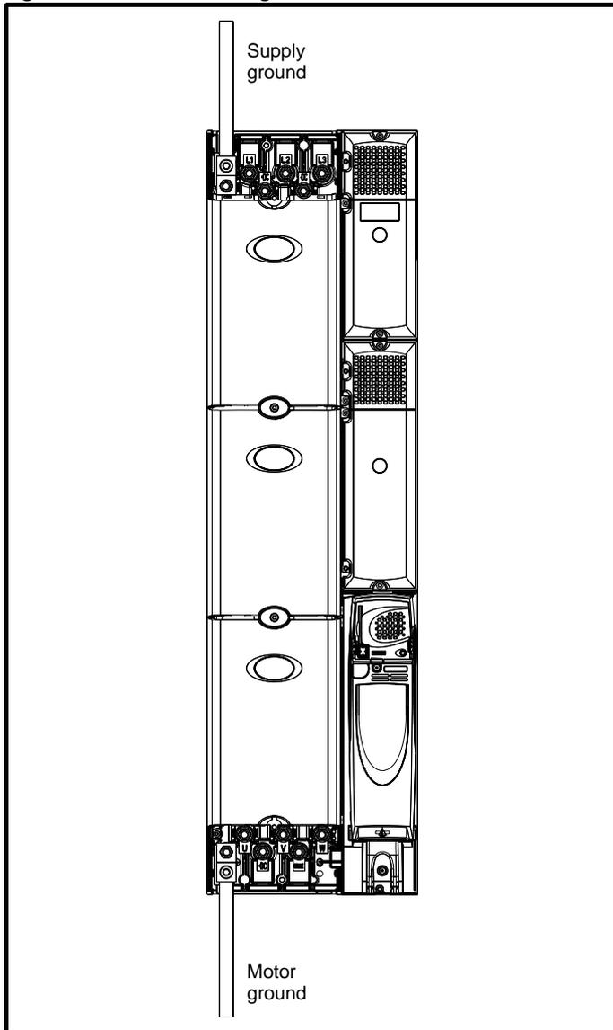
**Figure 6-4 Unidrive SPMD ground connections**
