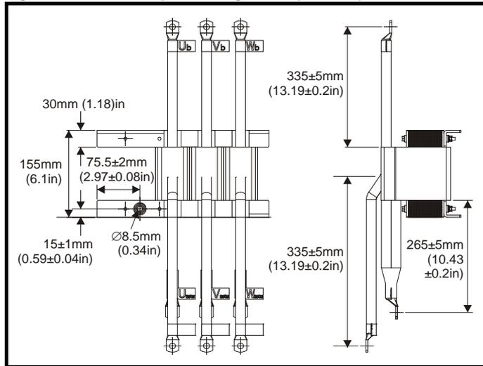
For overall dimensions and other details, refer to section 6.3 *Output sharing choke specification* on page 69.
