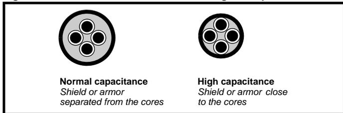
The cable used for Table 6-19 and Table 6-20 is shielded and contains four cores. Typical capacitance for this type of cable is 130pF/m (i.e. from one core to all others and the shield connected together).
