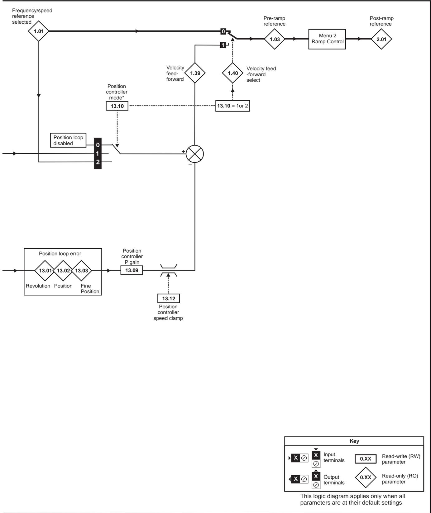
Figure 13-22 Menu 13 Closed-loop logic diagram
