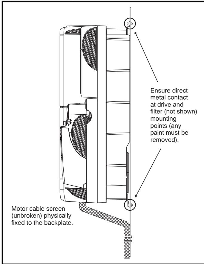
Connect the shield of the motor cable to the ground terminal of the motor frame using a link that is as short as possible and not exceeding 50mm (2in) long. A full 360° termination of the shield to the terminal housing of the motor is beneficial.
