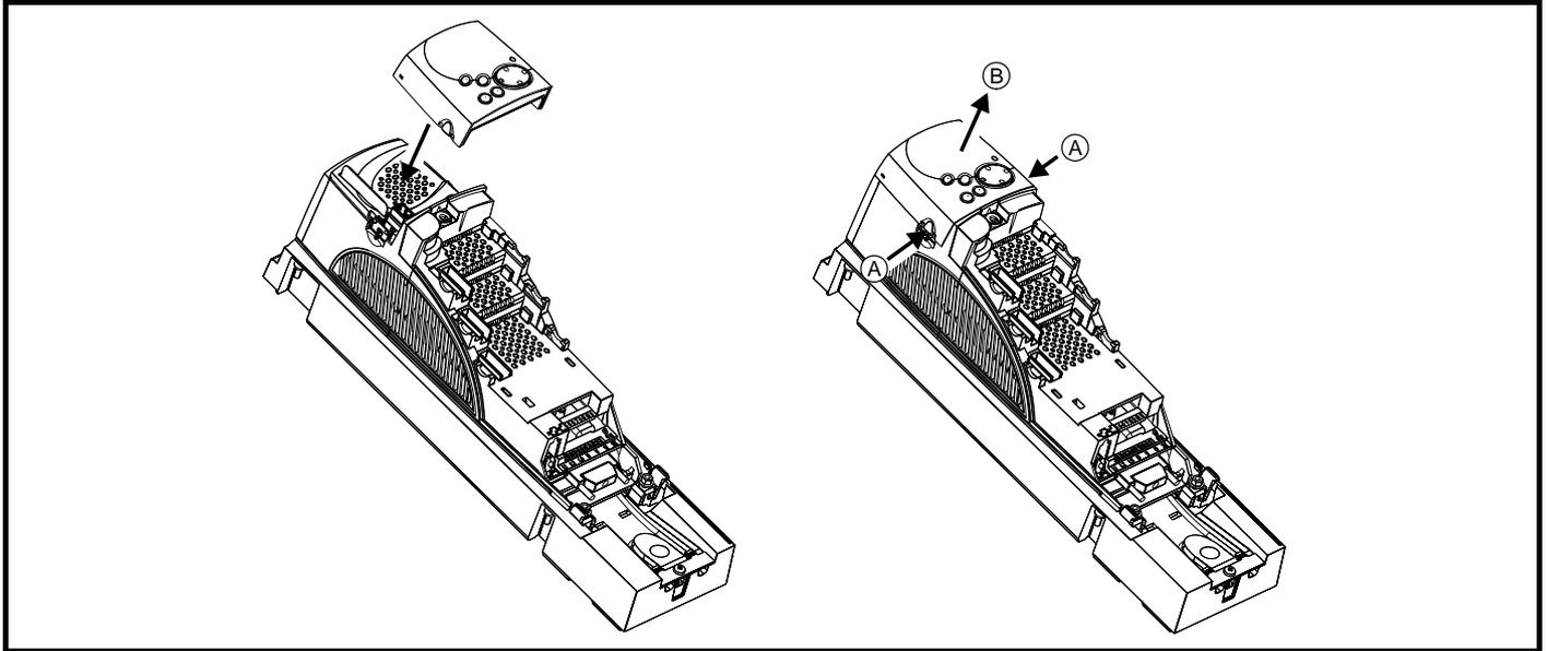
To install, align the keypad and press gently in the direction shown until it clicks into position.
