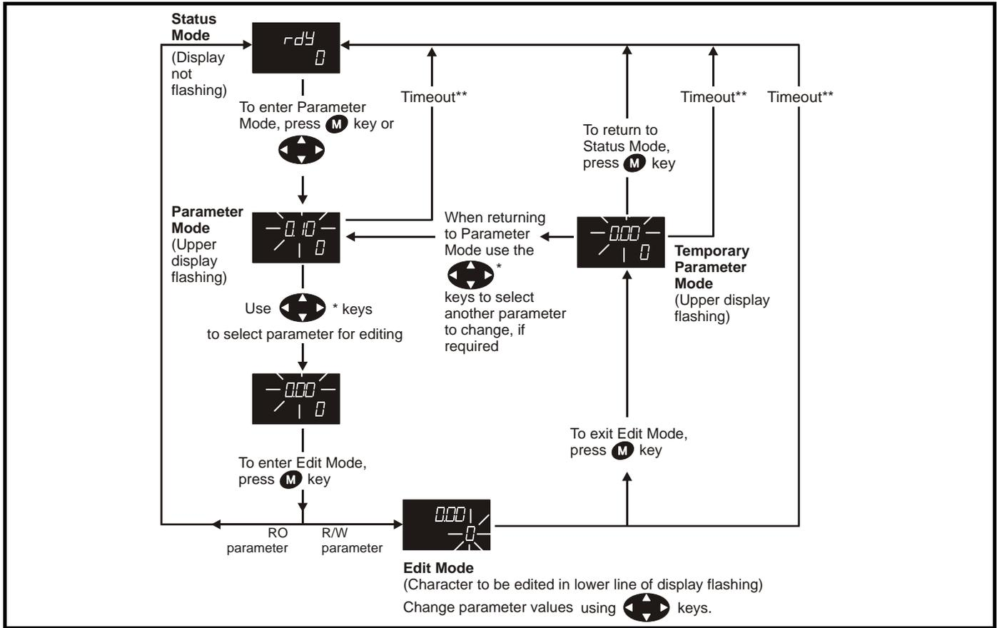
\* can only be used to move between menus if L2 access has been enabled (Pr 0.49). Refer to section 7.9 on page 106.
