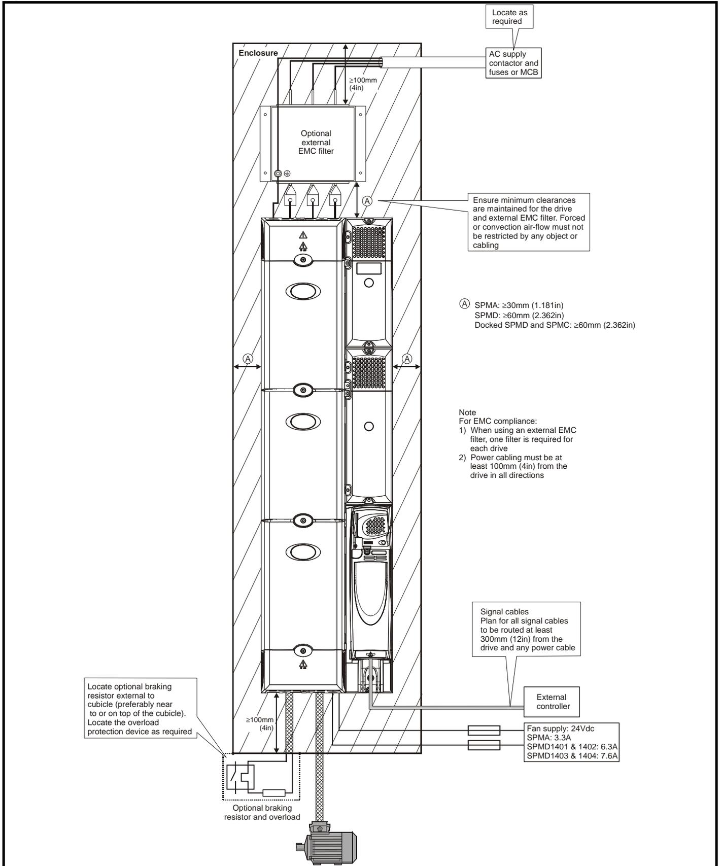
**Figure 5-28 Alternative enclosure layout: Undocked Unidrive SPMD and SPMC**
