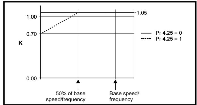
If Pr 4.25 is 0 the characteristic is for a motor which can operate at rated current over the whole speed range. Induction motors with this type of characteristic normally have forced cooling. If Pr 4.25 is 1 the characteristic is intended for motors where the cooling effect of motor fan reduces with reduced motor speed below 50% of base speed/frequency. The maximum value for  $K$  is 1.05, so that above the knee of the characteristics the motor can operate continuously up to 105% current.
