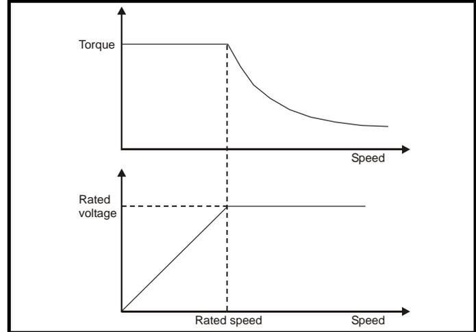
Care must be taken to ensure the torque available above base speed is sufficient for the application to run satisfactorily.
