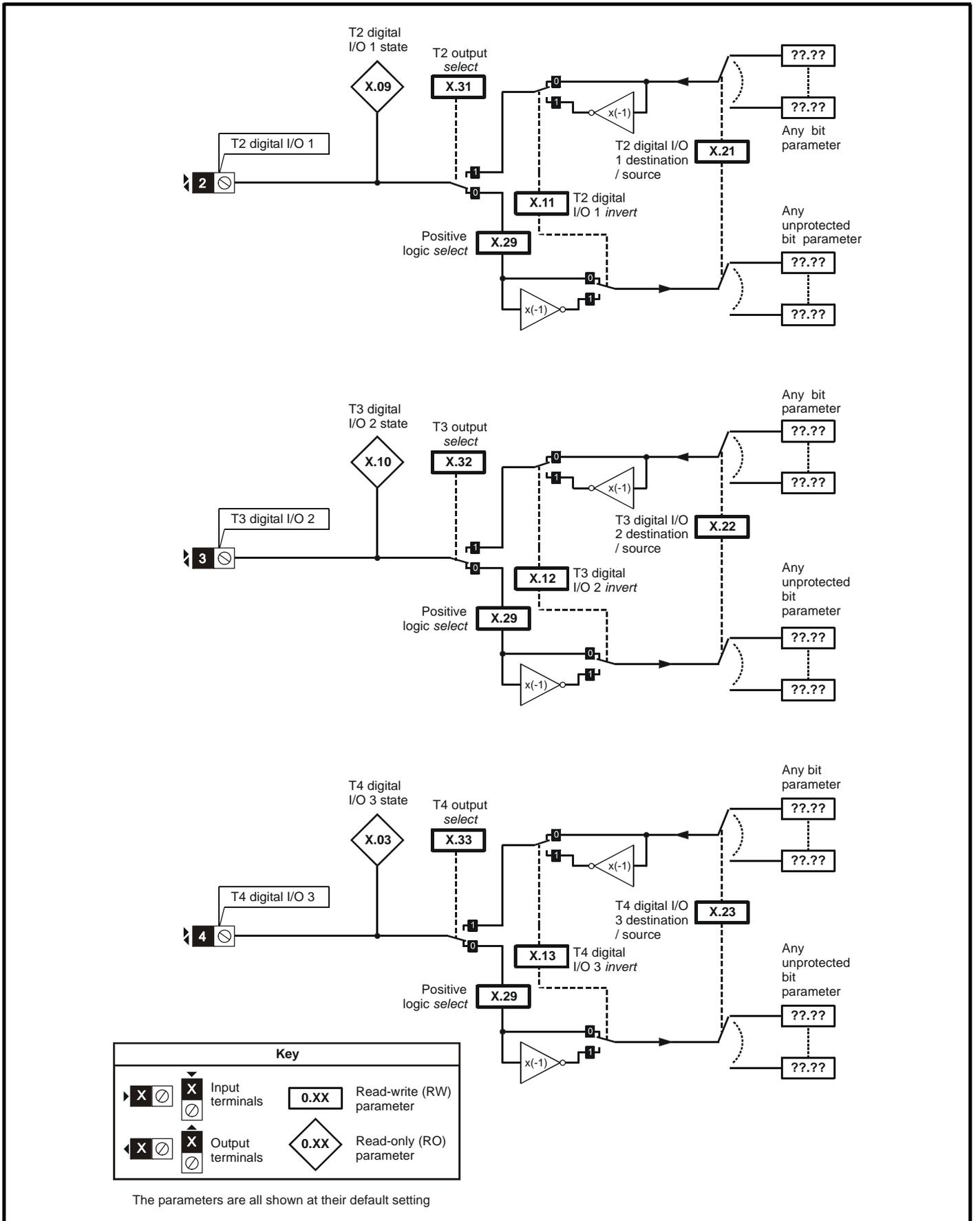
Figure 13-31 SM-I/O Plus digital logic diagram 2
