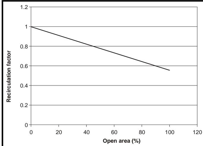
This is an approximation to the amount of air that is re-circulated within the enclosure due to inlet and outlet venting restrictions. The factor has a safety factor built in to it to ensure a safe result. The factor has been calculated using CFD software, testing the amount of heat flow back into the drive when different vent restrictions are given. The factor can also be applied to an SPMA and separated SPMD.
