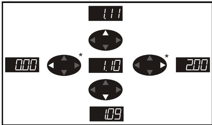
\* can only be used to move between menus if L2 access has been enabled (Pr 0.49). Refer to section 7.9 *Parameter access level and security* on page 106.
