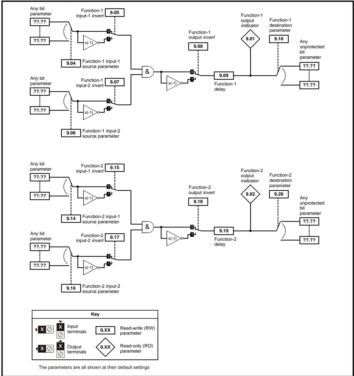
**Figure 13-14 Menu 9 logic diagram: Motorized pot and binary sum**
