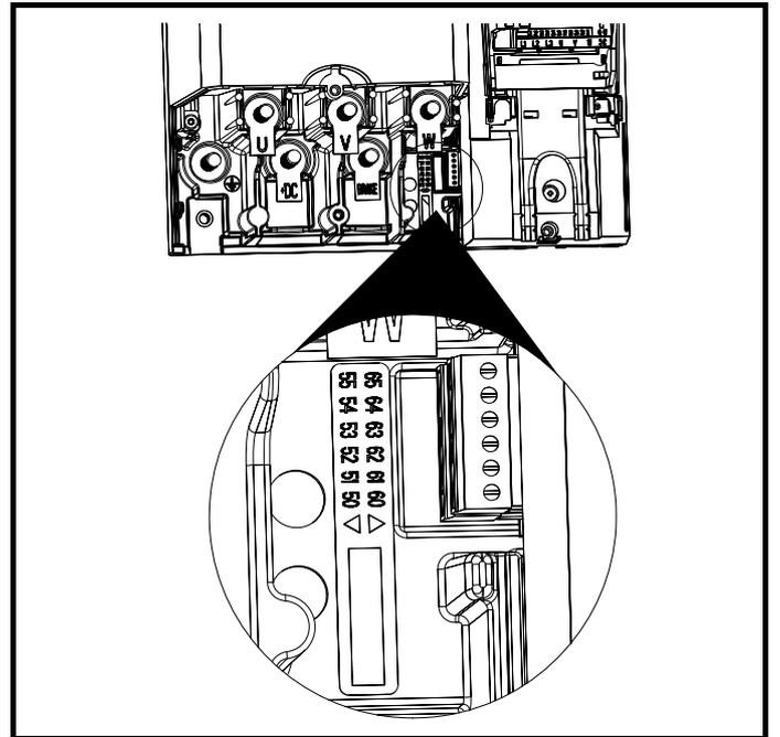
Figure 6-40 SPMA low voltage DC mode enable connections
