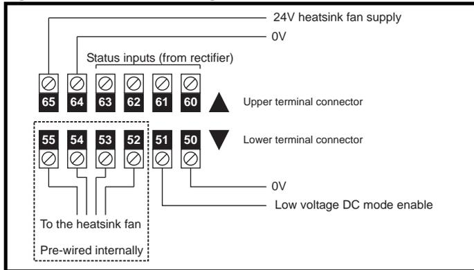
**6.15.1 Low voltage DC mode enable connections (SPMA/D)**
