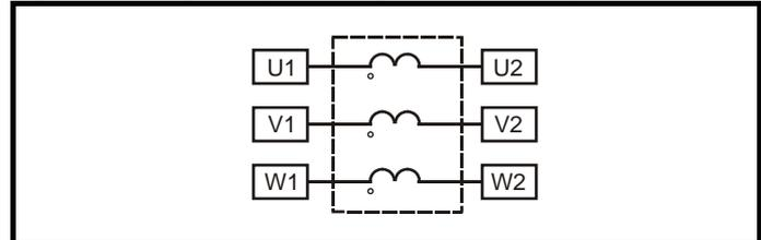
**Figure 2-10 Dual output sharing choke (OTLX1X)**
