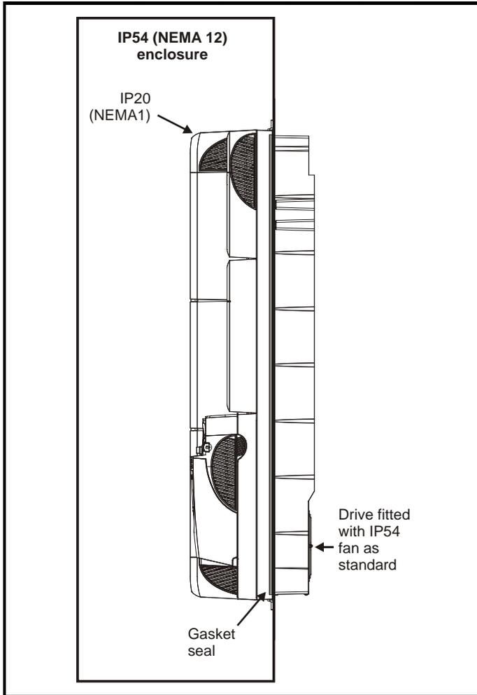
The main gasket should be installed as shown in Figure 5-39. Any screws / bolts that are used for mounting should be installed with the nylon washers provided in the kit box to maintain a seal around the screw hole. See Figure 5-40.
