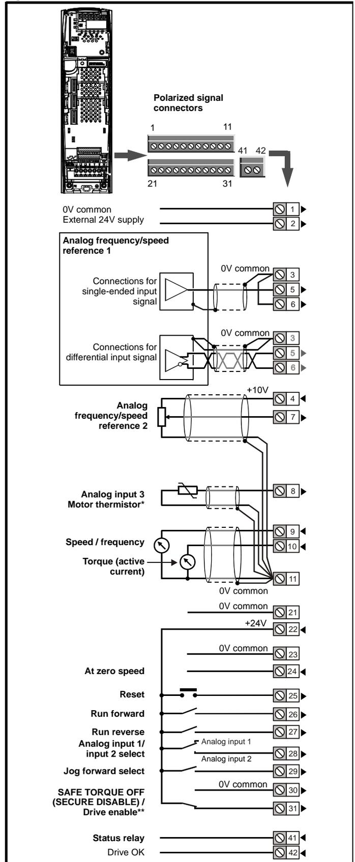
\* With software V01.07.00 and later, Analog input 3 is configured as a motor thermistor input. With software V01.06.02 and earlier, Analog input 3 has no default function. Refer to *Analog input 3* on page 94.
