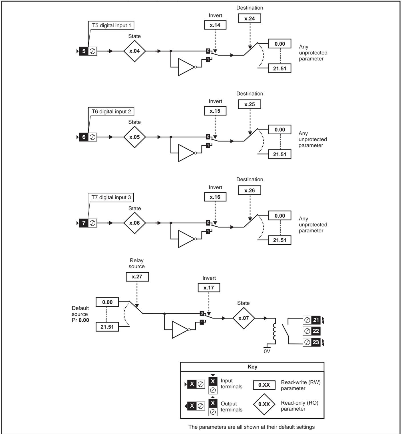
Figure 13-33 SM-I/O Lite & SM-I/O Timer analog I/O logic diagram
