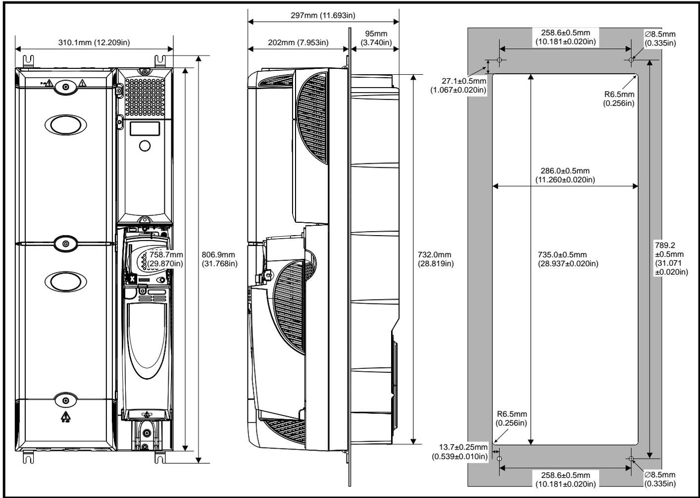
**Figure 5-20 Through-panel mounting the Unidrive SPMC/U (rectifier)**
