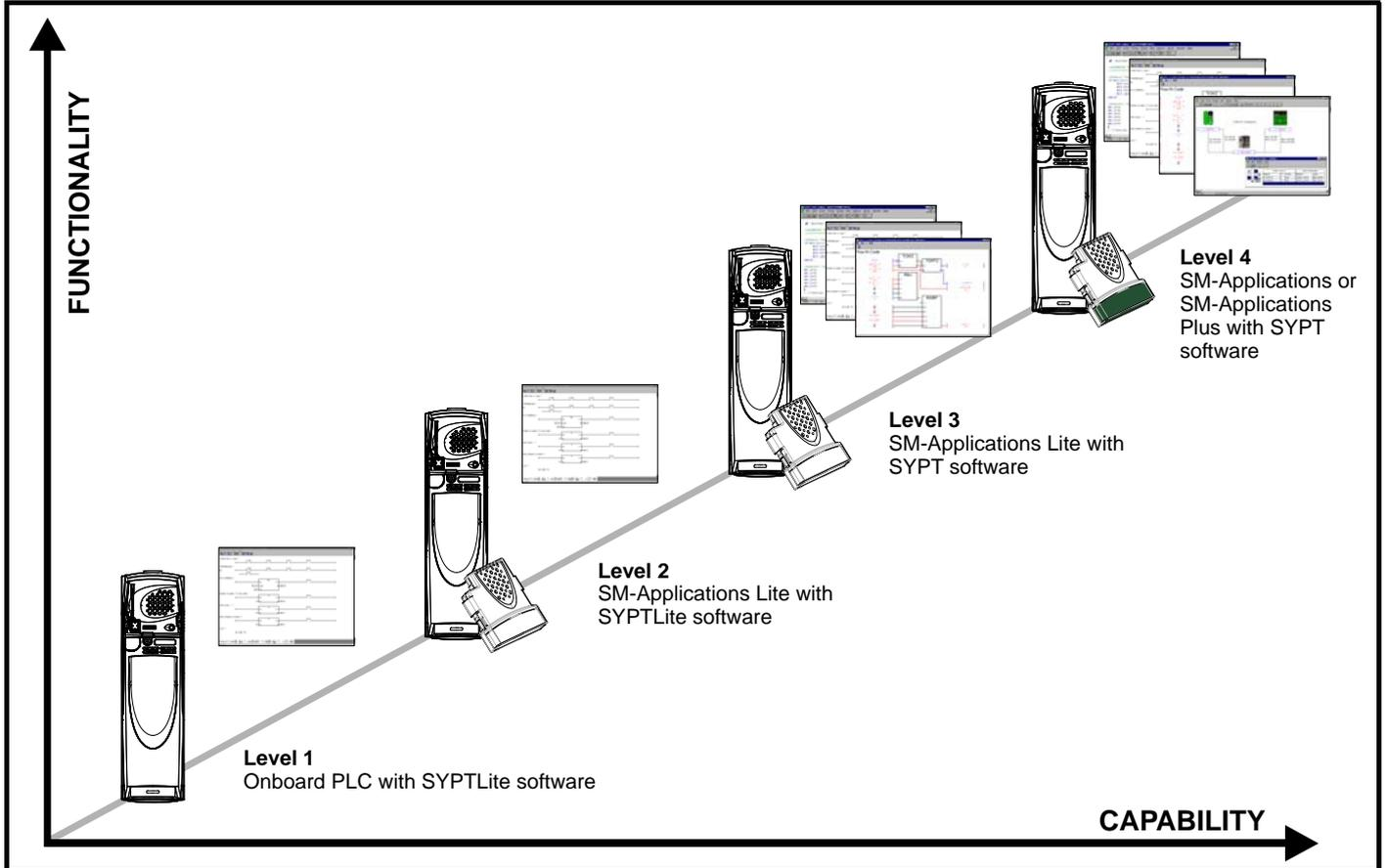
SYPTLite can be used with either the Onboard PLC in the Unidrive SP or with SM-Applications Lite to create ladder logic programs.
