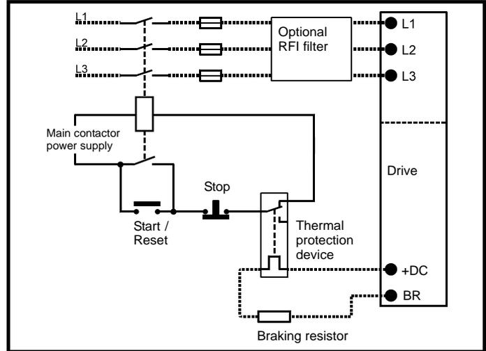
See Figure 6-1 and Figure 6-2 on page 65 for the location of the +DC and braking resistor connections.
