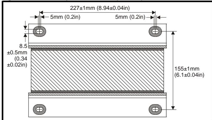
Figure 5-47 Single line input reactor force cooled (INLX0XW)
