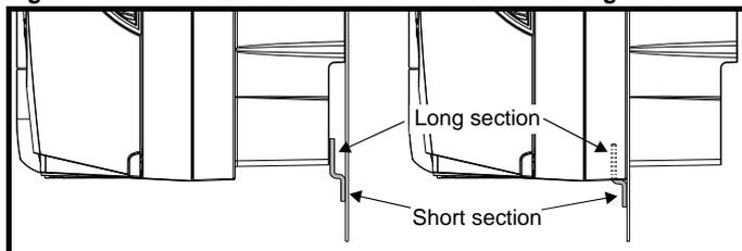
When through-panel mounted, the mounting brackets on the left hand side of the Unidrive SPMA and SPMD can be secured using the screws already located there. This only applies to the bottom of the Unidrive SPMC/U rectifier.
