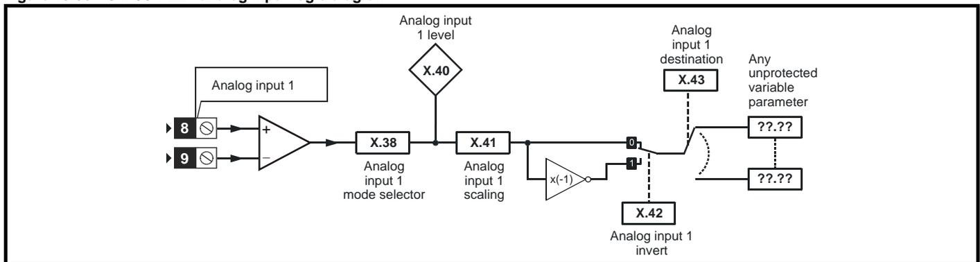
**Figure 13-39 SM-I/O PELV analog output logic diagram**
