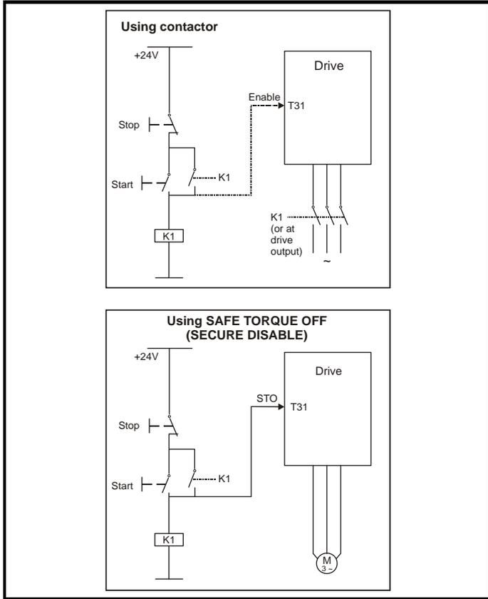
In the second example, illustrated in Figure 6-46 and Figure 6-47, a conventional high-integrity system which uses two safety contactors with auxiliary contacts with connected movement is replaced by a single SAFE TORQUE OFF (SECURE DISABLE) system. This arrangement meets EN954-1 category 3.
