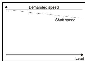
In order to prevent the speed droop shown above slip compensation should be enabled.
