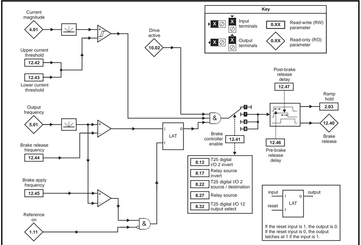
**Figure 13-18 Open-loop brake sequence**
