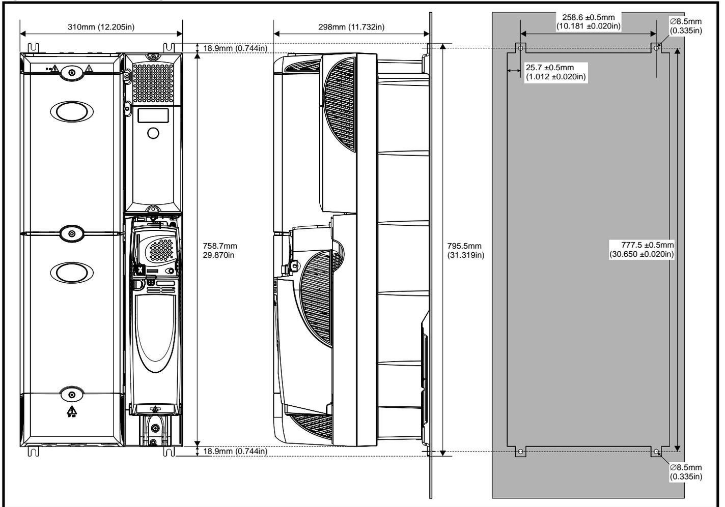
**Figure 5-16 Surface mounting the Unidrive SPMC/U (rectifier)**
