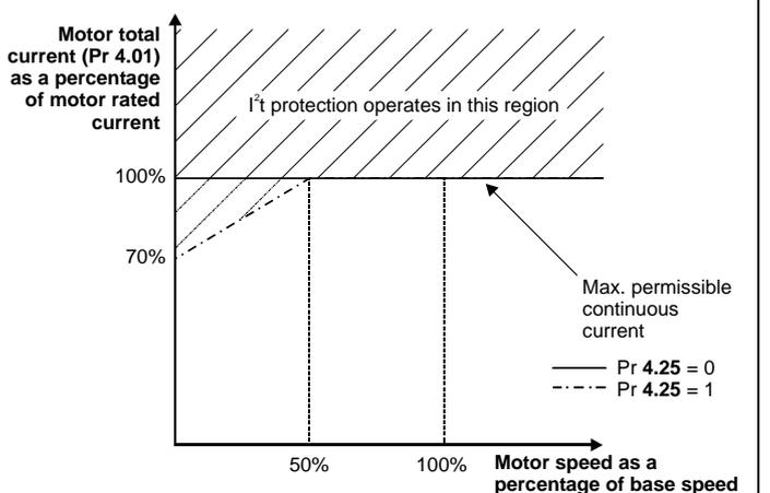
The continuous current ratings given are for maximum 40°C (104°F), 1000m altitude and 3.0 kHz switching. Derating is required for higher switching frequencies, ambient temperature >40°C (104°F), high altitude and parallel applications. For further information, refer to section 14.1.1 *Power and current ratings (Derating for switching frequency and temperature)* on page 263.
