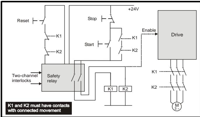
The safety function of the example circuit is to ensure that the motor does not operate when the interlocks are not signalling a safe state. The safety relay is used to check the two interlock channels and detect faults in those channels. The stop/start buttons are shown for completeness, they do not carry out a safety function and are not necessary for the safe operation of the circuit
