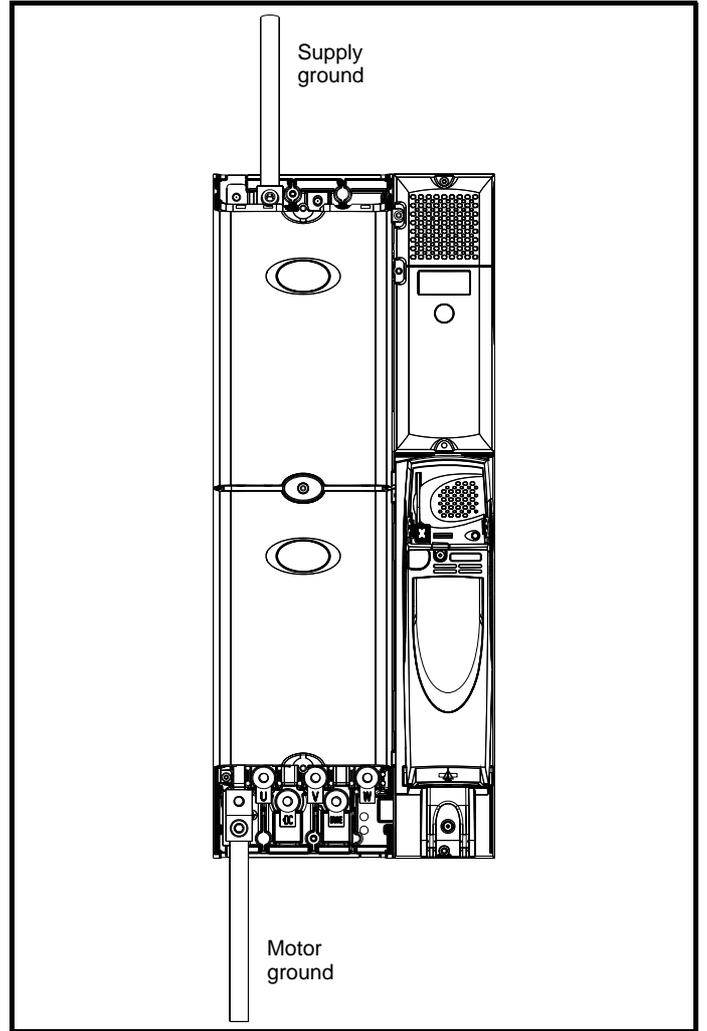
**Figure 6-5 Unidrive SPMC/U ground connections**
