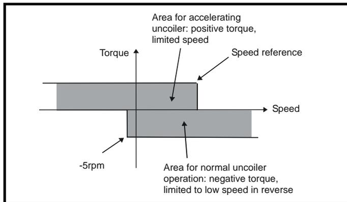
**4: Speed control with torque feed-forward**
