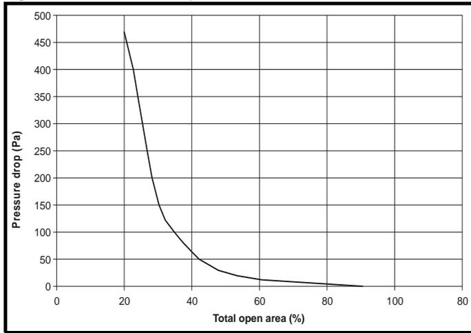
**Best practice:** Size the enclosure air inlet and exit vents at least as large as the venturi opening of the fan used. This will ensure a negligible back pressure.
