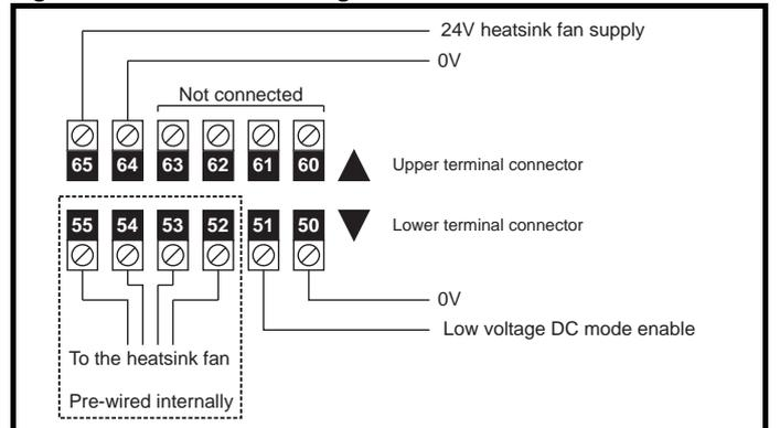
**Figure 6-41 SPMD low voltage DC mode enable connections**
