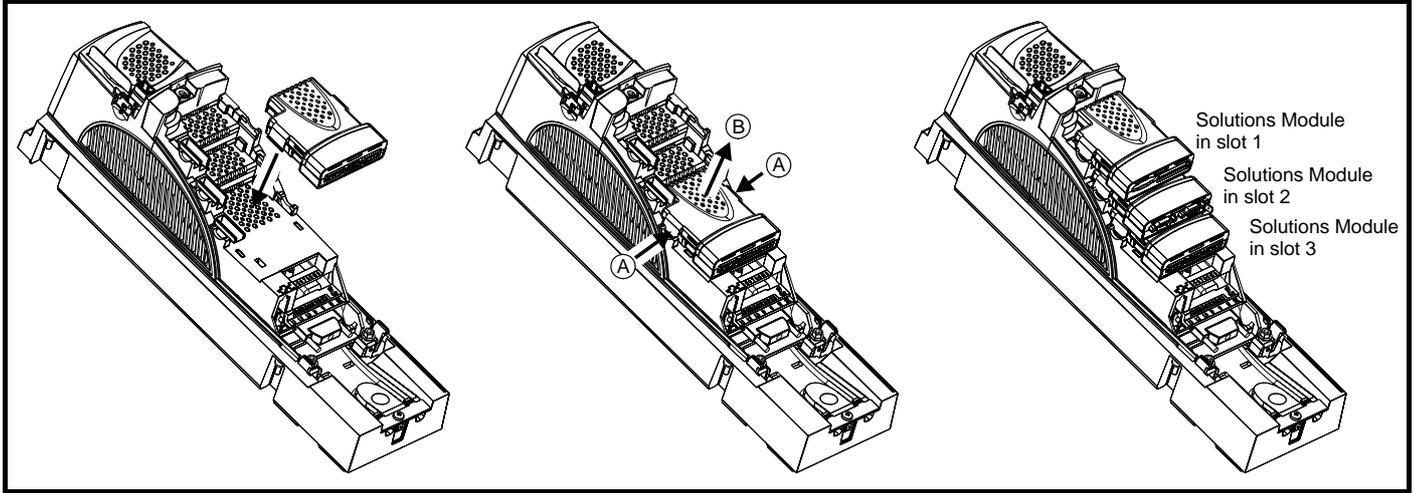
To install the Solutions Module, press down in the direction shown above until it clicks into place.
