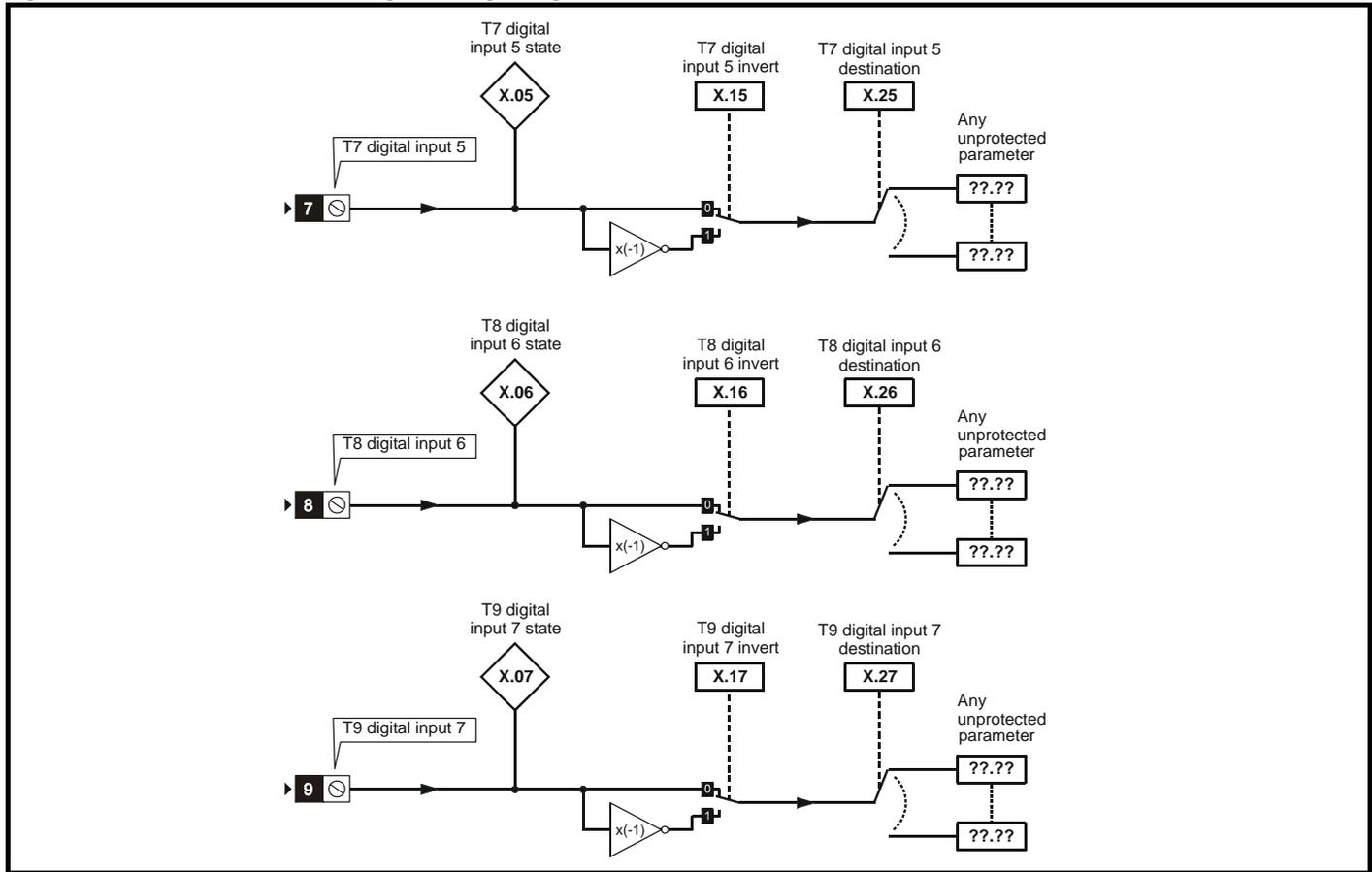
**Figure 13-42 SM-I/O 24V Protected relay logic diagram**
