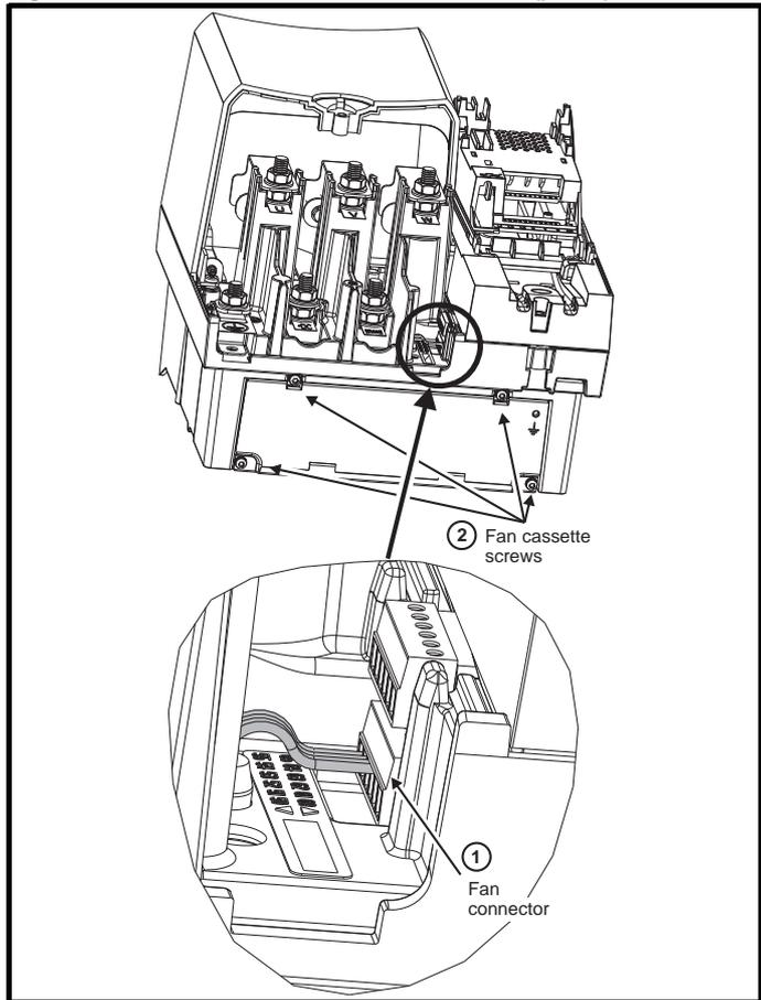
**Figure 5-37 Removal of Unidrive SPMA/D fan (part 2)**
