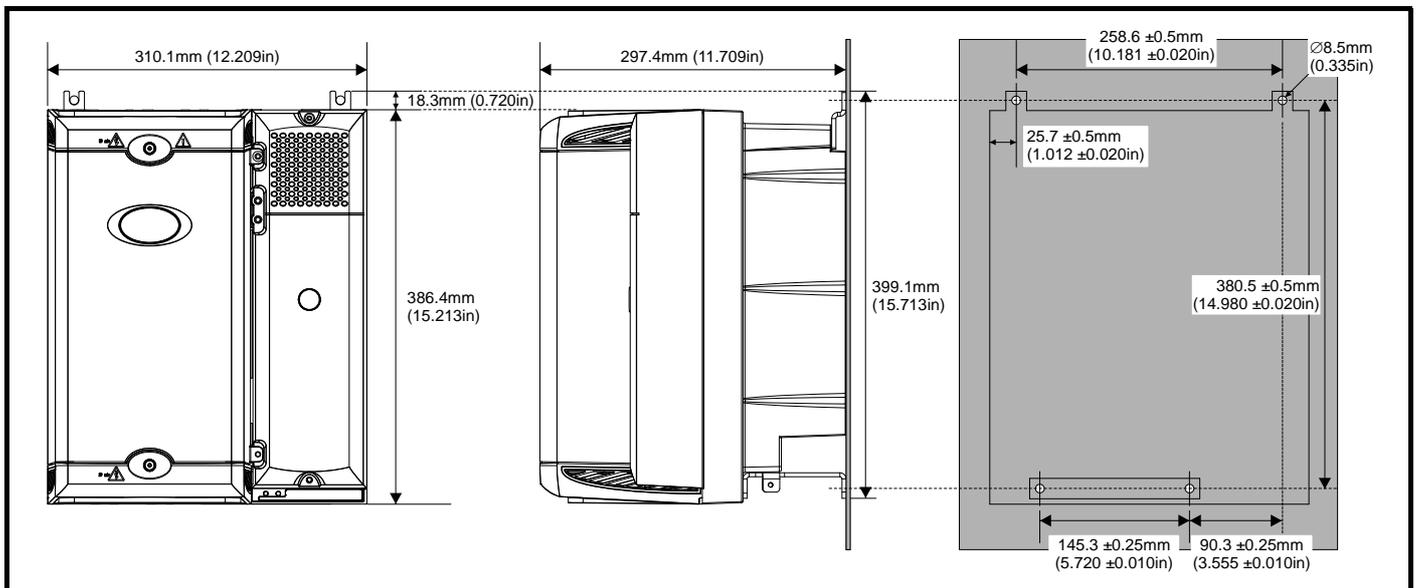
**Figure 5-17 Surface mounting the Unidrive SPMD with SPMC/U (rectifier) and docking kit**
