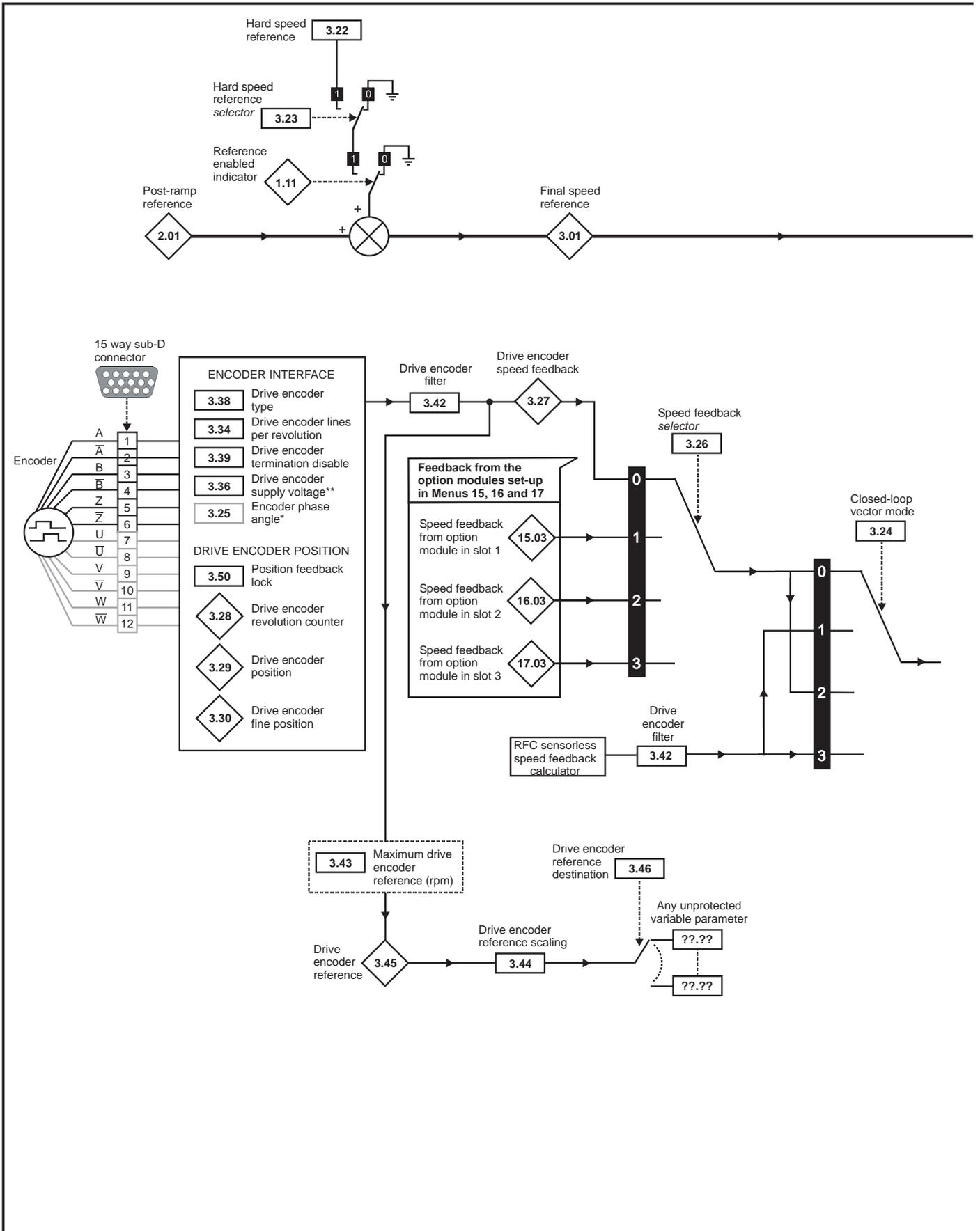
**NOTE** \*\*If output voltage from the encoder is >5V, then the termination resistors must be disabled Pr 3.39 to 0.
