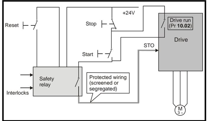
In the conventional system, a contactor failure in the unsafe direction is detected the next time the safety relay is reset. Since the drive is not part of the safety system it has to be assumed that AC power is always available to drive the motor, so two contactors in series are required in order to prevent the first failure from causing an unsafe event (i.e. the motor driven).
