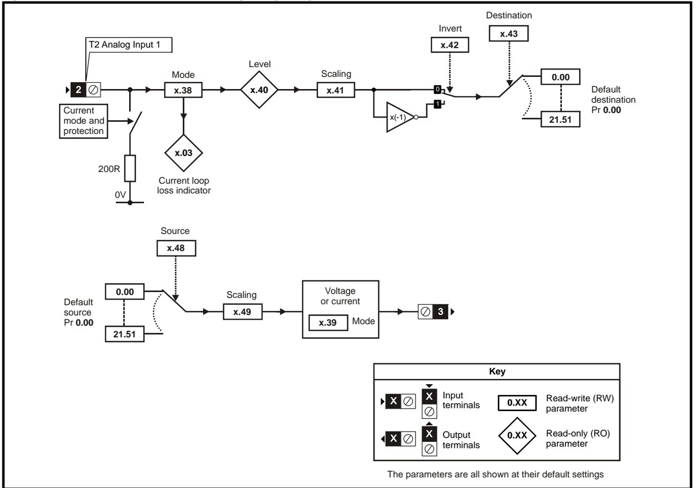
Figure 13-34 SM-I/O Timer real time clock logic diagram
