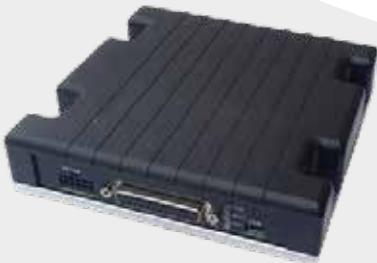
Our Medium Power Dual Channel, Motor Controllers, have advanced core technology, multiple connectivity options and scripting support. Up to 2 x 60A. Conduction cooling plate with ABS plastic cover. Supports trapezoidal commutation and sinusoidal mode with field oriented control.
