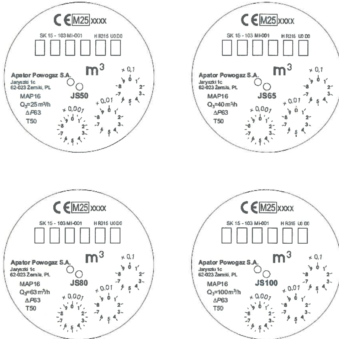
Fig. 6a: Illustrative view of dial and marking of the water meters JS (samples for R315)
